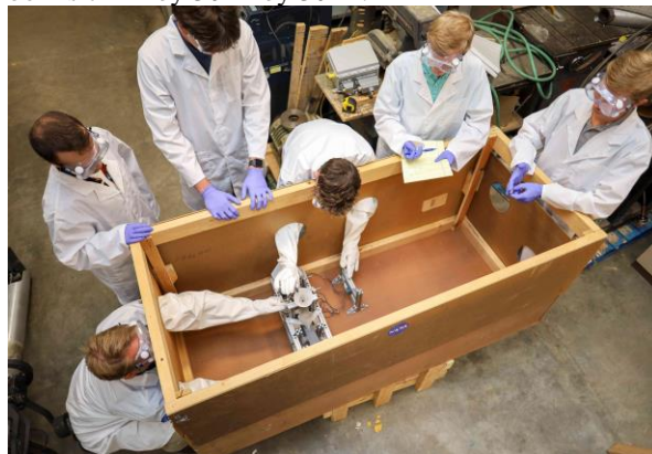
Figure 3. Team rehearsing in-flight operation for parabolic flight testing with a wood mock-up glovebox.
